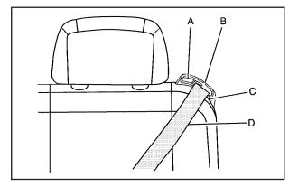
1. Slide the edge of the safety belt (D) through the opening at the top of the guide (B).
